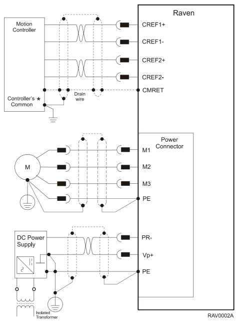
\* The controller common must be connected to the CMRET whenever the common mode difference is over 6V.
